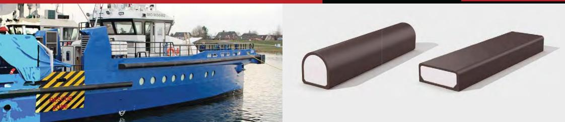
Polyurethane is increasingly used for the production of fenders as it provides a number of advantages over rubber. Polyurethane is extremely durable, it has lower friction and lower specific gravity. The material is also non-marking and it can be produced in various striking colours.
