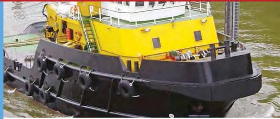
W fenders are designed for use in extreme conditions and to absorb excessive bumps and knocks. This type of fender is very suitable for application on the bow and stern of tugs, workboats and icebreakers. The grooves on the top of the fender provide extra grip and low pressure while pushing. With two flexible legs also allow for easy installation of the W fender with a large or small radius by means of guide rods.
