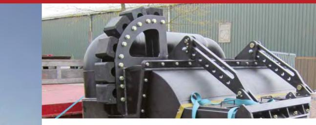
Strong rubber fenders can prevent damage in rough conditions or in the event of a collision between the drag head and the hull of the ship. These fenders are used in different versions, to prevent damage to the hull of the ship, the drag head and the gimbal ring.
