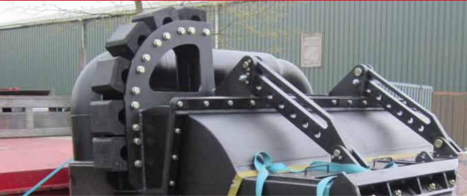
Strong rubber fenders can prevent damage in rough conditions or in the event of a collision between the drag head and the hull of the ship. These fenders are used in different versions, to prevent damage to the hull of the ship, the drag head and the gimbal ring.
